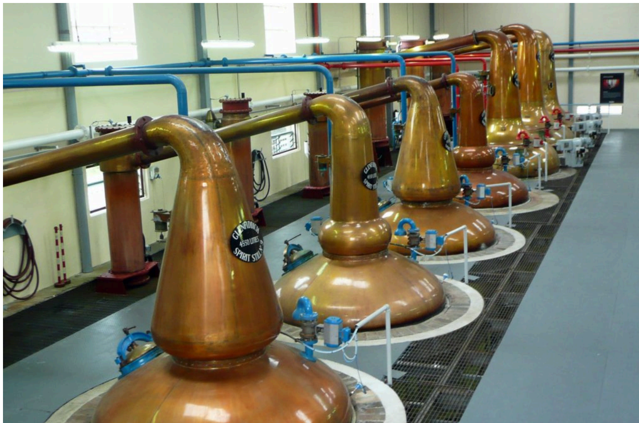
Figure 6: The copper stills at the Glenfiddich Distillery in Scotland
