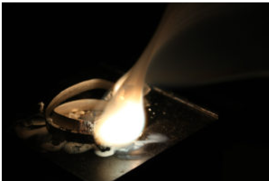
Figure 4: Burning magnesium to form magnesium oxide is an example of a chemical change
