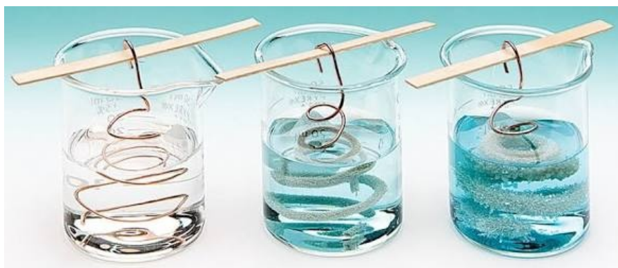
Figure 12: The precipitation reaction between silver nitrate and copper
