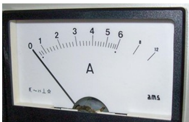
Figure 3: An ammeter and a circuit diagram showing the symbol for an ammeter
