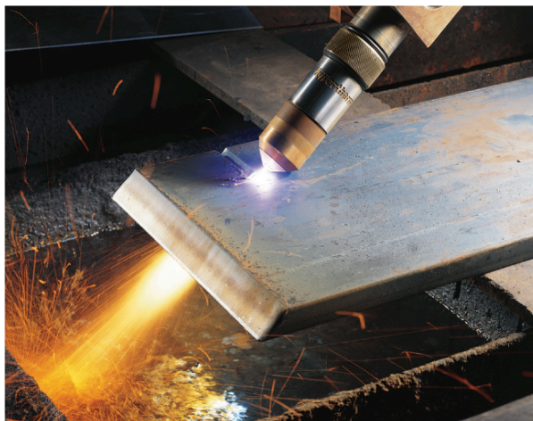
Figure 3: A plasma torch being used to cut metal
